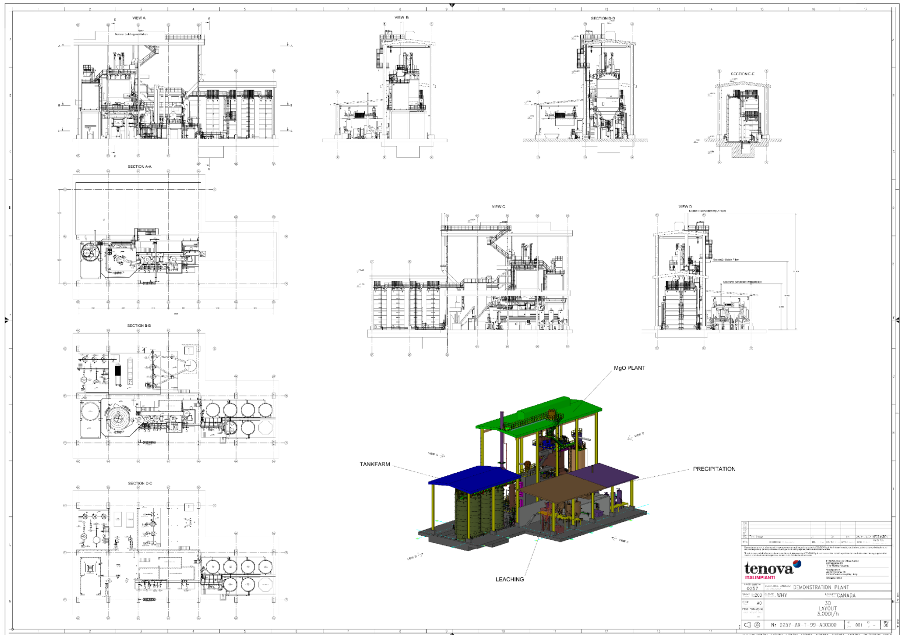
Figure 5: General Layout of Demonstration Plant – Equipment.
