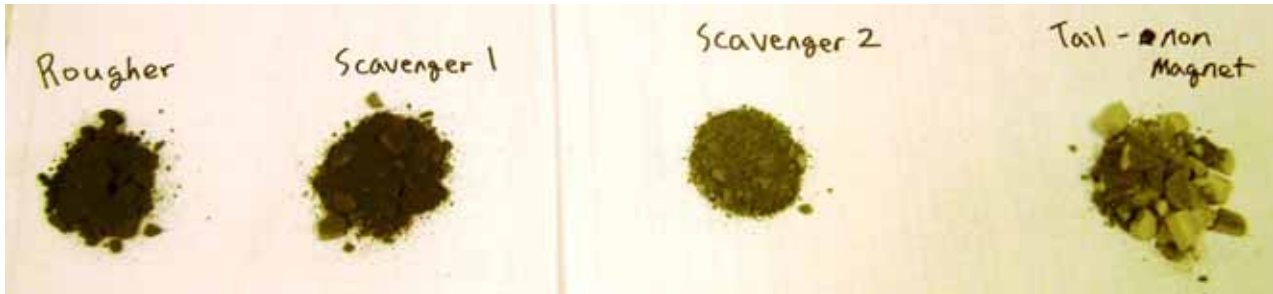
Figure 1: View of the different magnetic separation product. Note the darker colour of the rougher and scavenger 1.
